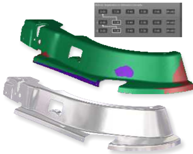
Compensation of the D20 operation based on springback measured after the trimming operation – results are 90% within the tolerance level.
