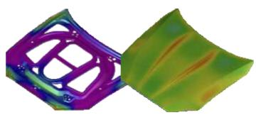
New Target for Hood Inner after Compensation
