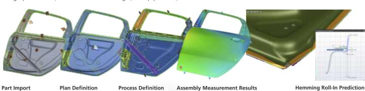
quickly evaluate alternative part and assembly process designs, identify the causes of dimensional deviations and undertake effective countermeasures. With AutoForm Assembly, assembly process issues can be successfully resolved prior to the start of production.
